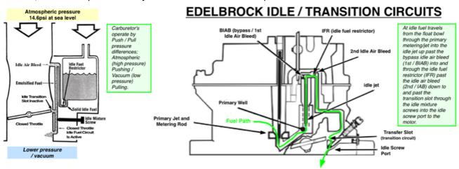
Notice as the throttle opens, the transition slot predominately supplies the fuel to the motor.
