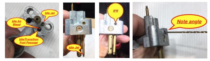
The IFR will need to be drilled to except the tubing, select a drill bit slightly smaller than the tubing (needs to be a tight fit). Using our example IFR size above, we'll drill it with a #53 bit increasing the IFR size to .0595, slightly smaller than the 1/16" tubing's outside diameter .0625). Using a #50 drill bit slightly chamfer the IFR opening to allow the tubing to insert.
