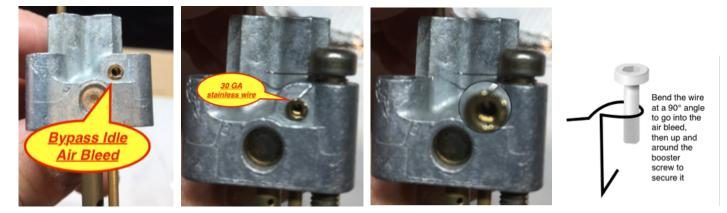
Put the carburetor back together. Warm the motor up completely (motor must be completely at operating temperatures and the choke off), re-adjust idle mixture screws (this is necessary due to the increased fuel supply). Take it for a test drive, noting air fuel ratios and performance changes in transition circuit at off idle up to 2000rpm (in gear on the road). Keep a log of all changes and their outcomes.
