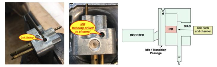
Spray carburetor cleaner through the IFR passage and through the air bleeds followed with compressed air to clean out any drill shaving or debris.
