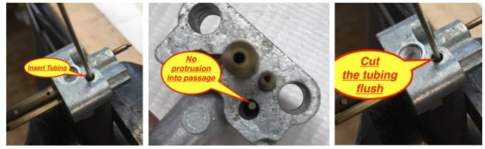
Using a drill bit slightly larger than the tubing, drill the tubing down through the bypass air bleed hole until the tubing is flush to the IFR channel watching frequently while drilling to prevent drilling into the IFR channel. Once drilled flush to the channel, continue drilling a little more to slightly chamfer the tubing's inside edge into channel (allows a smooth fuel flow).
