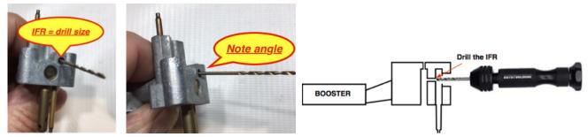
After drilling, spray carburetor cleaner liberally through the IFR and air bleed passages followed with compressed air to remove any drilling debris.
