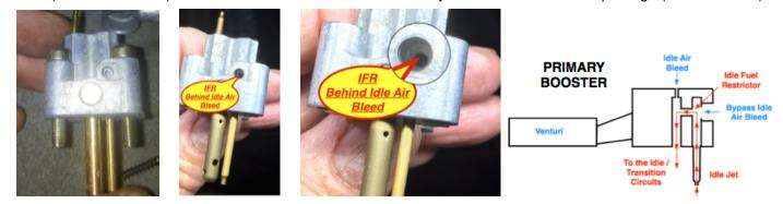
Before you start drilling it is important to determine the size of the IFR in your carburetor first. This is done by using a numbered drill bit set. It is important to use numbered drill bits, numbered drill bits are smaller than standard bits and their incremental sizing is much closer together. Start with a #55 bit and gently insert the drill bit's shank (non drilling end of the bit) into the IFR hole, increase / decrease the drill bit size until it fits the hole exactly and document the size.
