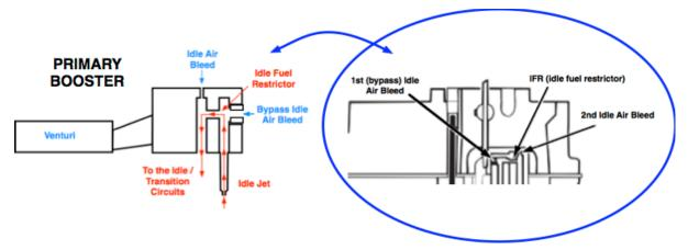
**To restrict the BIAB**, simply place a small piece of 28-30 gauge stainless jewelry wire into its orifice. The wire placed in the BIAB orifice obstructs it slightly causing a restriction to the air flow entering which in turn creates more siphon action at the idle jet, bringing more fuel to the IFR and a richer mixture.
