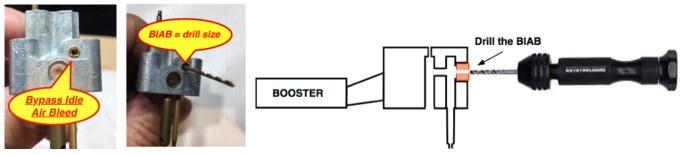
After drilling, spray carburetor cleaner liberally through the IFR and air bleed passages followed with compressed air to remove any drilling debris. Put the carburetor back together and test.
