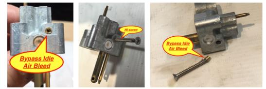
With the plug removed you'll be able to see a small hole inside behind where the air bleed was, the small hole inside is the IFR (idle fuel restrictor). The IFR is the channel between the idle jet and the idle/transition passage (see illustration).
